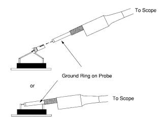
Ripple and Noise will be measured with a scope and 20 MHz bandwith. Since most scopes are able to track a far higher frequency it is necessary to manually reduce the bandwidth internal to the oscilloscope. Bandwidth-limiting at the oscilloscope is preferable to a hardware-based limitation.
