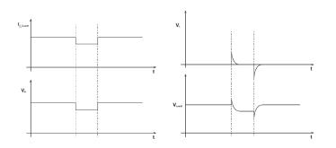
Fig. 2a: Load jump caused by the first load Fig. 2b: Input voltage at the second load in the event of a load jump
