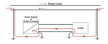
Fig. 4: A DC load is connected via a long line to the power supply unit. The neutral lines of the AC mains supply network are typically earthed at both the power supply and the load in according with applicable installation rules.
