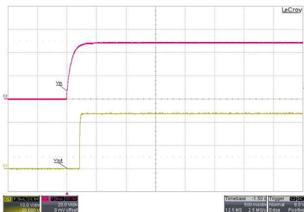
Typical Input Start-Up and Output Rise Characteristic V_{in} = V_{in nom} ; Full Load
