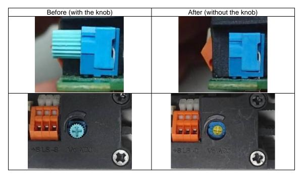
By removing the knob, the height for adjusting the output voltage decreased by about 5 mm. A screwdriver can still be used for output voltage adjustment; there is only a change in appearance.
