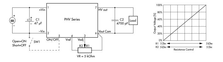
Connection for remote control voltage control
