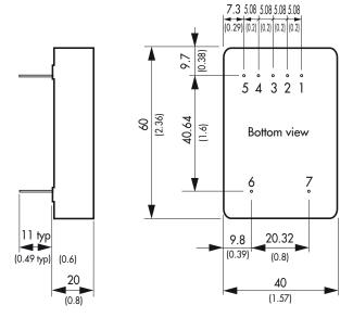
Dimensions in [mm], () = Inch Pin diameter: 0.8 ±0.05 (0.03 ±0.002) Tolerances: ±0.5 (±0.02)
