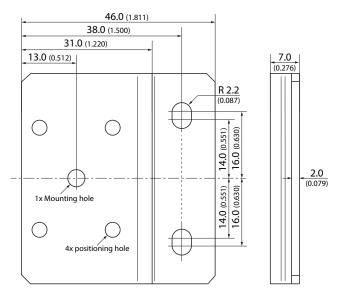
All dimensions in mm (inch) Tolerance:  $\pm 0.3 (\pm 0.012)$
