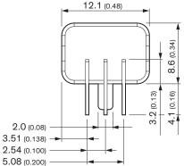
Dimensions in mm (inch) Tolerances: x.xx  $\pm 0.5$  ( $\pm 0.02$ ) Tolerances: x.xxx  $\pm 0.25$  ( $\pm 0.01$ ) Pin pitch tolerances:  $\pm 0.10$  ( $\pm 0.04$ )
