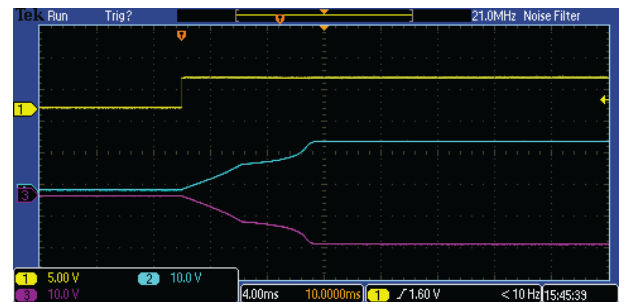
Typical Start-Up and Output Rise Characteristic
