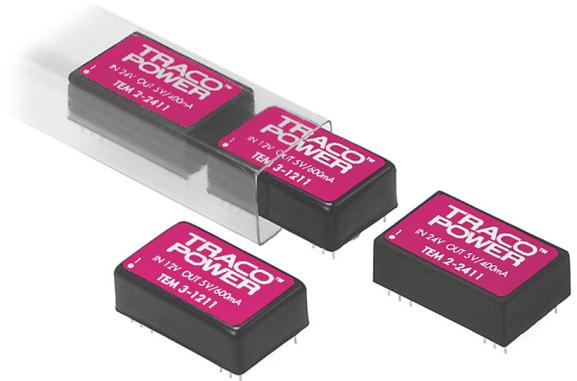
The TEM 2 series is a family of isolated dc/dc converters in a DIP-24 package. They offer tight line/load regulation and 1000 VDC I/O isolation. Standard features include an internal filter to reduce reflected input ripple current and to guarantee low output noise. This product series provides a cost effective solution by many industrial or consumer electronics applications.
